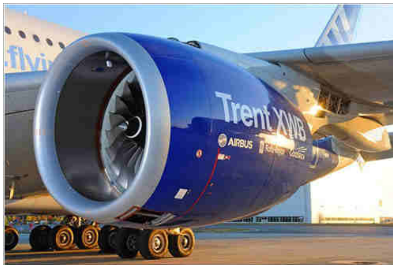
Classic Trent engine, with shrouded fan
